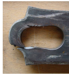
(a) bearing failure A1212_2
