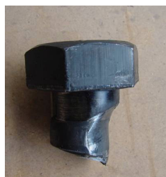
(a) bolt deformation
