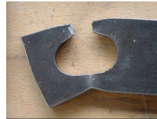
Fig. 5 – Failure of the inner plates of the test joint of specimens A1212_2 and A1210_2
