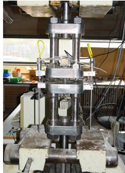
(b) LVDT on opposite sides of the equipment.
