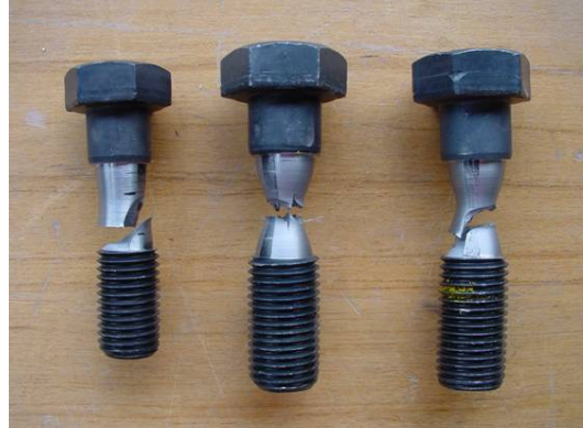
Figure 6.5 – Comparison of the necking on the three groups of specimens (from the left to the right: M24 10.9, M27 8.8, and M27 10.9).
