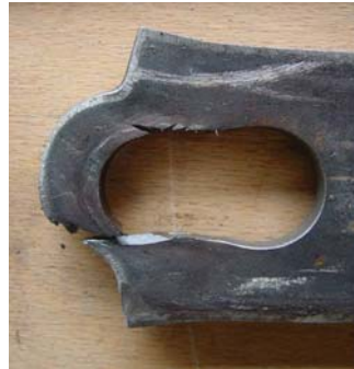
(a) bearing failure mechanism A1212_2
