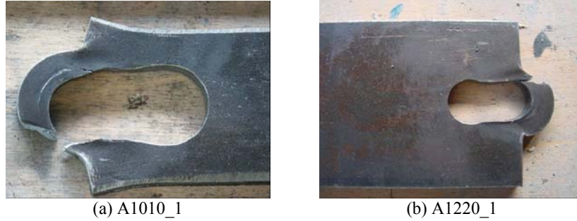
Figure 7.7 – Shear fracture with splitting and without splitting present on test specimens A1010_1 and A1220_1, respectively.
