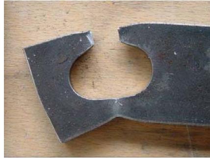
(b) net section failure mechanism A1210_2
