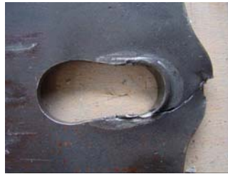
Figure 7.8 – Shear and tensile fracture present on test specimen A2020_1
