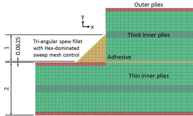
Figure 4: Zoom on fillet region and material section assignments (dimensions in mm)
