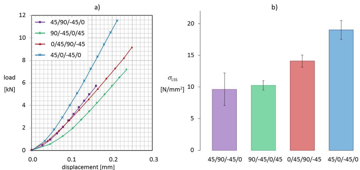
Figure 6: a) Load-displacement curves, b) average lap shear strength and corresponding standard deviation for different layups
