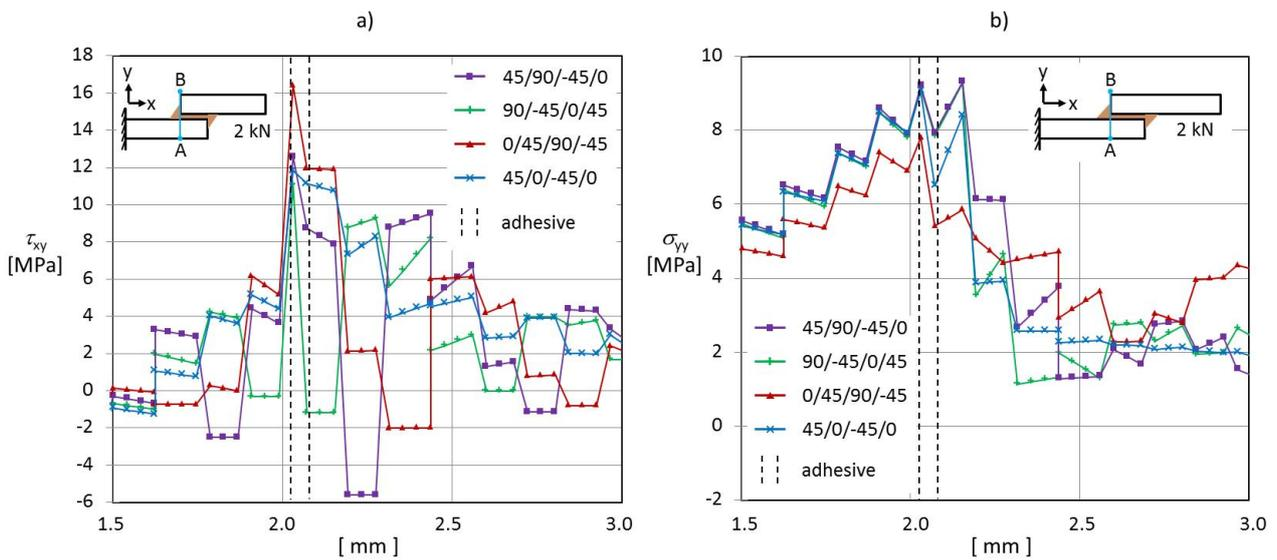
Figure 12: Shear ( $\tau_{xy}$ ), a) and peel ( $\sigma_{yy}$ ), b) stress through the overlap thickness at centre position in width, focused region around the bond line
