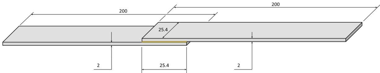
a) SLJ specimen design (dimensions in mm)
