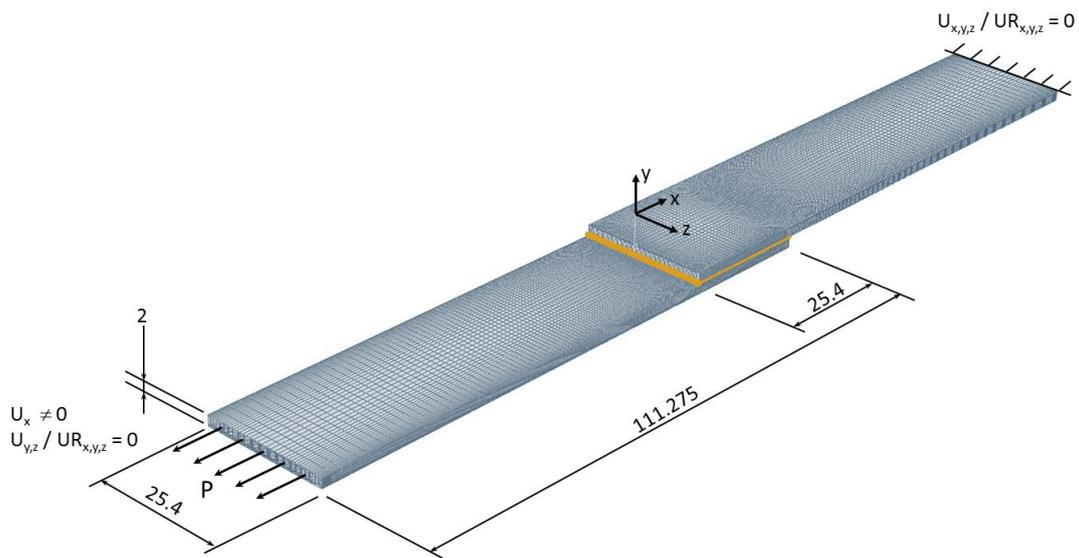
Figure 3: 3D FE-model between the clamps with specimen dimensions and boundary conditions (dimensions in mm)
