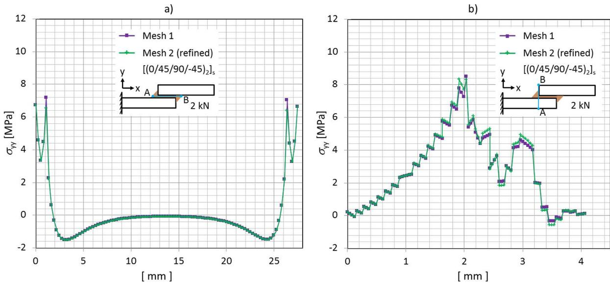
Figure 5: Mesh convergence study on peel stress ( $\sigma_{yy}$ ) distribution along overlap length a) and through bond line thickness b)
