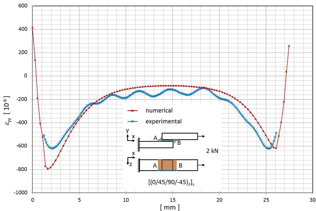
Figure 9: Peel strain( $\epsilon_{yy}$ ) in microstrain  $[10^{-6}]$  along the bond line, numerical versus experimental method
