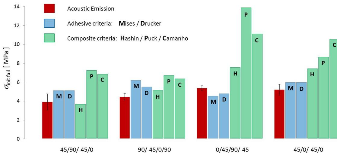
Figure 13: Average lap shear stress at damage initiation: experimental versus numerical results
