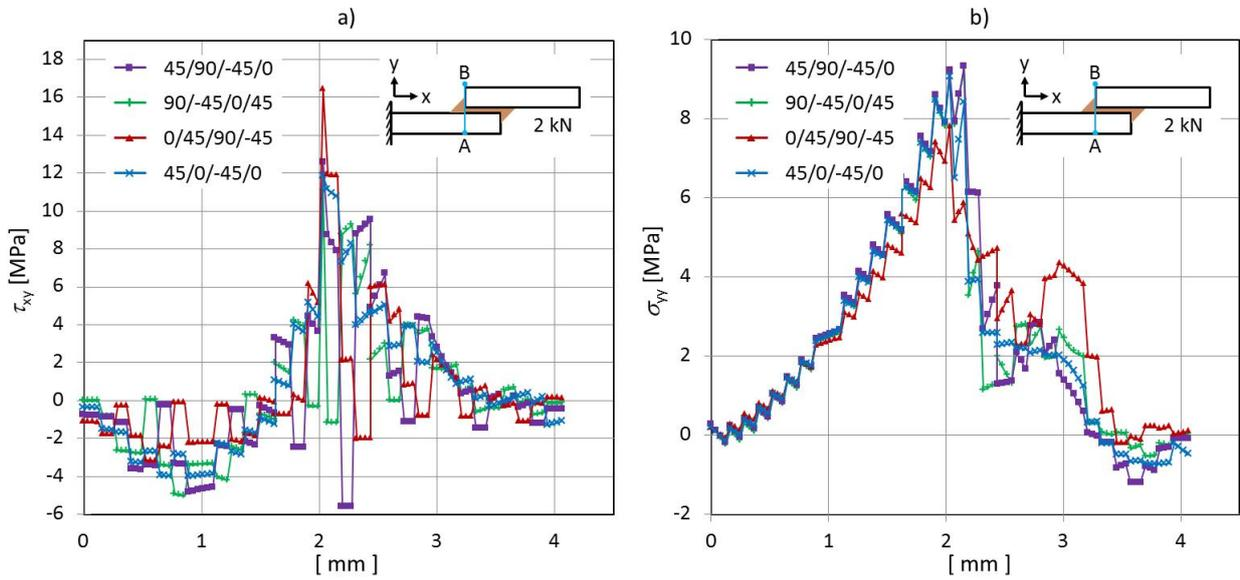
Figure 11: Shear ( $\tau_{xy}$ ), a) and peel ( $\sigma_{yy}$ ), b) stress through the overlap thickness at centre position in width
