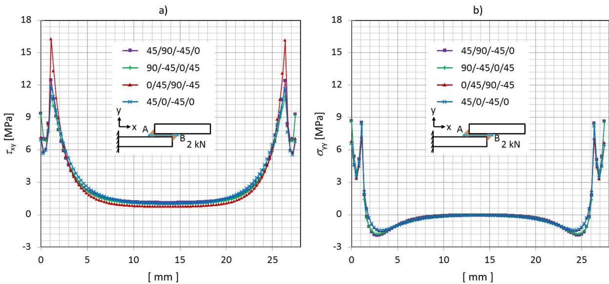
Figure 10: a) Shear ( $\tau_{xy}$ ), and b) peel ( $\sigma_{yy}$ ), stress along the bond line of the joint at centre position in width
