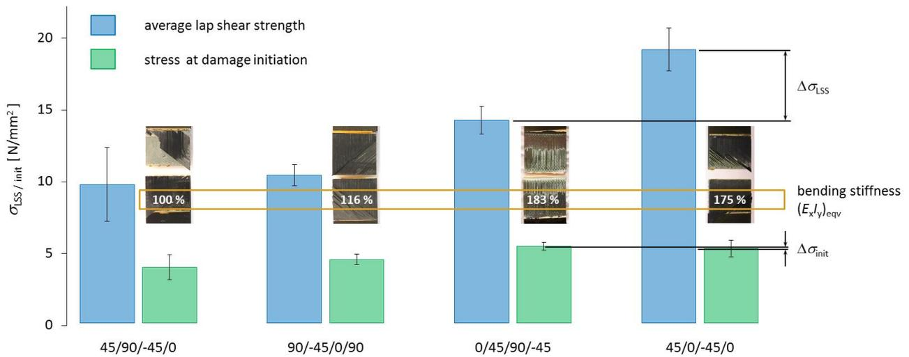
Figure 15: Average lap shear strength ( $\pm$  standard deviation) at maximum load vs. damage initiation in respect to bending stiffness
