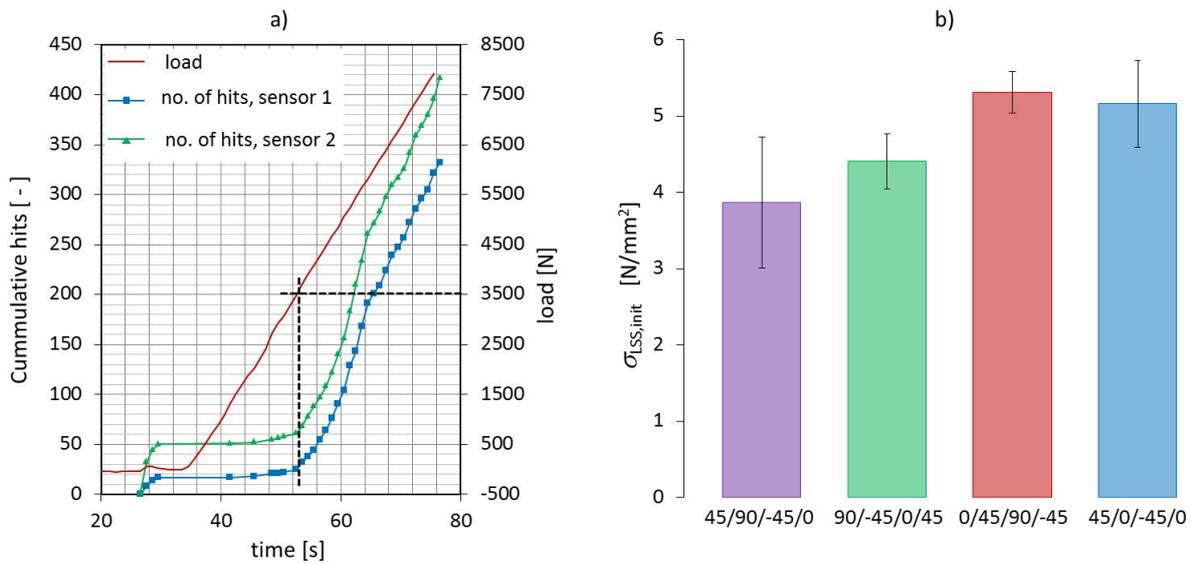
Figure 8: a) Cumulative acoustic hits vs. load for  $[(0/45/90/-45)_2]_s$ , b) average lap shear stress ( $\pm$  standard deviation) at damage initiation of different layups
