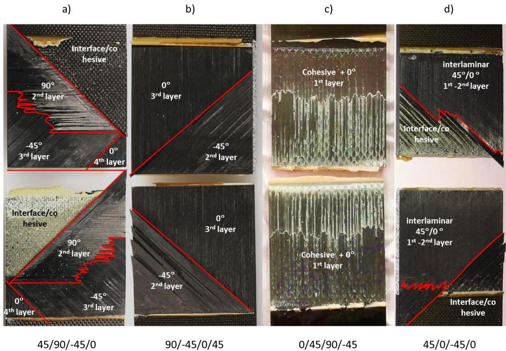
Figure 7: Typical fracture surfaces for each layup configuration
