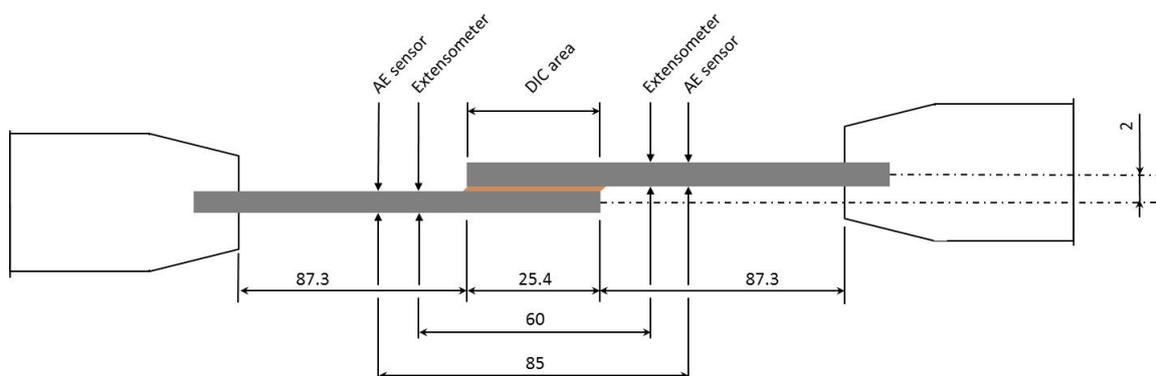
Figure 2: Test setup for static tensile loading (dimensions in mm)
