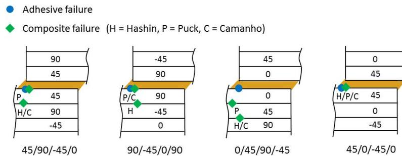
Figure 14: Location of damage initiation due to FEM-analysis
